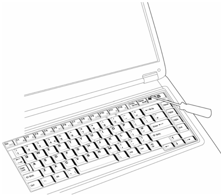
Figure 4-14 Removing the strip cover
